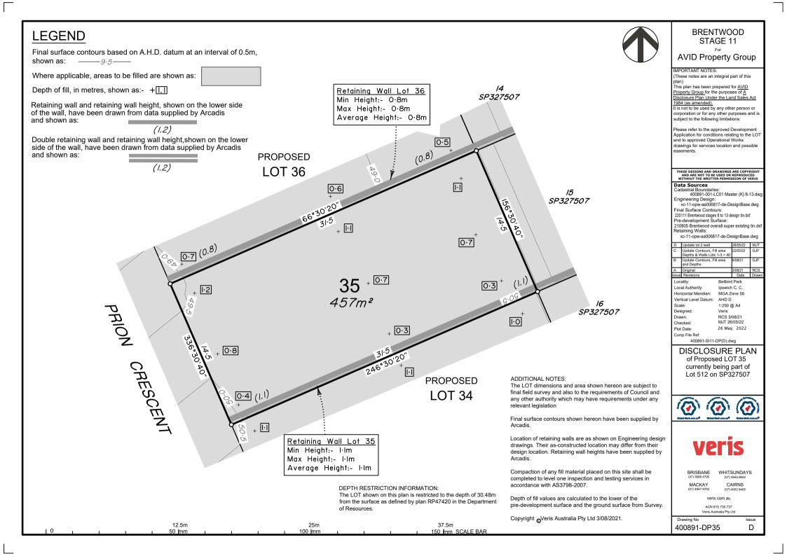
**BRENTWOOD LEGEND** STAGE 11 Final surface contours based on A.H.D. datum at an interval of 0.5m, **AVID Property Group** Where applicable, areas to be filled are shown as: (These notes are an integral part of this This plan has been prepared for AVID Depth of fill, in metres, shown as:- + []. Property Group for the purposes of A /3 Disclosure Plan Under the Land Sales Act Retaining wall and retaining wall height, shown on the lower side 1984 (as amended).
